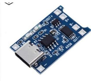
Gambar 7 Battery Charger Module [5]
