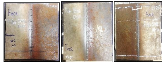
Gambar 3. Test Coupon (100A, 120A, 140 A)
