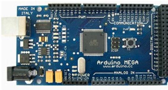
Gambar 4. Arduino Mega
