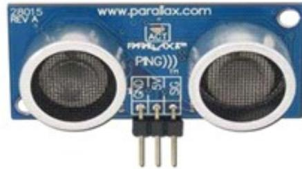
Gambar 2. Sensor Ultrasonic
