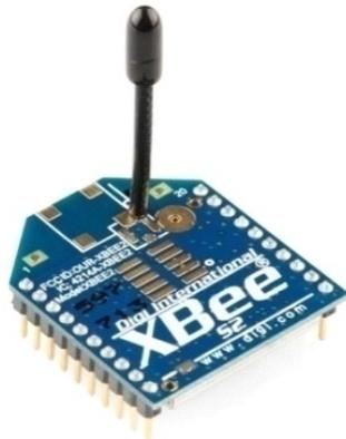
Gambar 6. Xbee Seri 2 Wire Antenna
