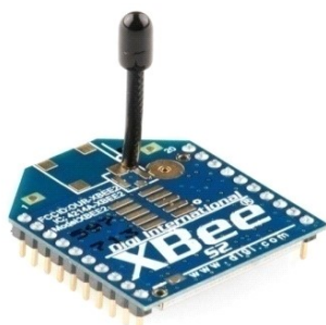
Gambar 2.6 : XBee Seri 2 Wire Antenna
