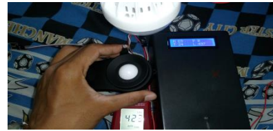
Gambar 4. Pengujian Intensitas Cahaya Lampu LED
