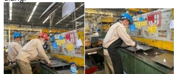
Gambar 4. Set Up Mesin Shearing dan Proses Shearing
