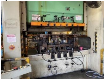
Gambar 5. Set Up Dies Stamping
